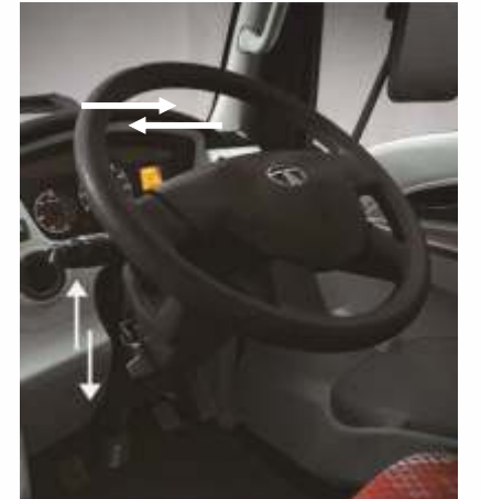
Tilt & telescopic steering for superior driving comfort
