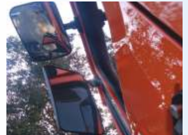
Side close proximity mirror Normal rear view mirror Wide angle rear view mirror
