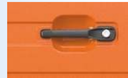
Single locking system for entire vehicle
