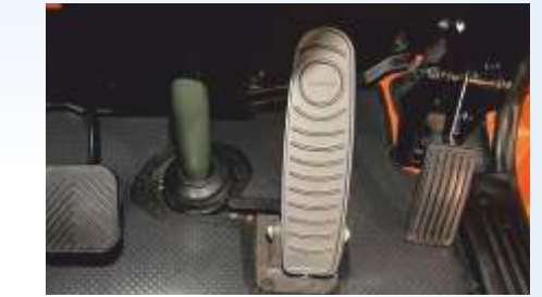
Pendant type accelerator and clutch pedal for fatigueless driving
